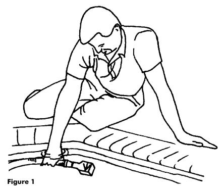
**If the flow is in the low range,** review the installation procedures. A dirty pool filter, clogged baskets and improperly set valves are usually the main cause of low flow. Other types of hydraulic problems may require a professional pool repairman.
