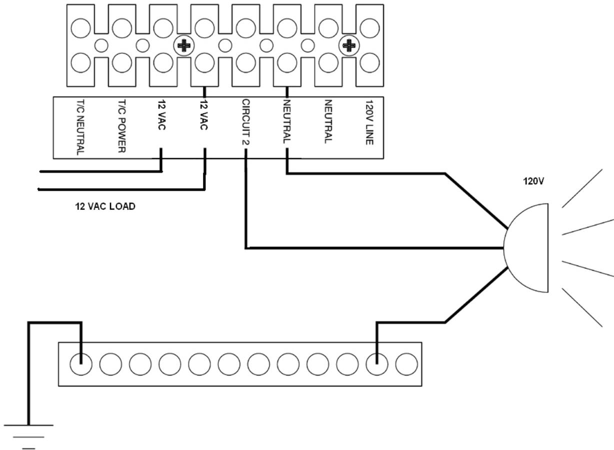
If this product is used to connect underwater lights directly, refer to 1999 NEC 680-21(b), 2002 NEC 680-24(b) or CEC 68-060, 062 and 066 for details.
