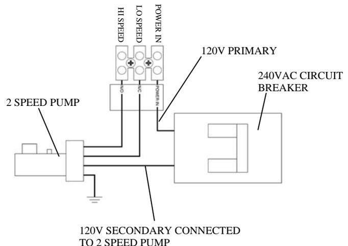
**NOTE: The Secondary 120V must be directly connected to the pump for 240V operation.**
