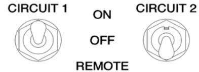
**NOTE: Circuit 1 is in the ON position and Circuit 2 is in the REMOTE position**
