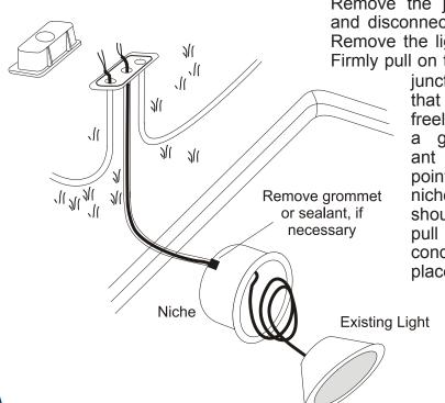
Remove the junction box cover and disconnect the existing light. Remove the light from the niche. Firmly pull on the light cord at the
