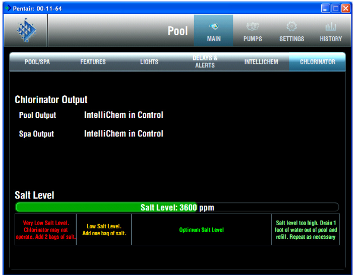
Chlorinator (IntelliChlor) with IntelliChem controller screen
