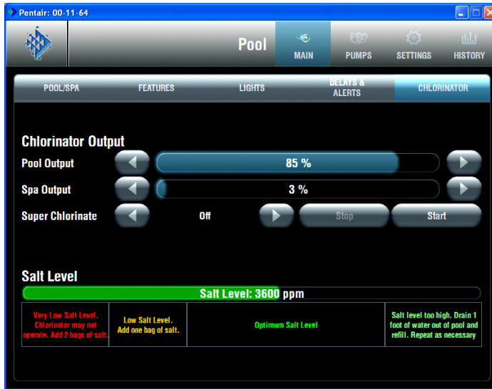
Chlorinator (IntelliChlor) screen
