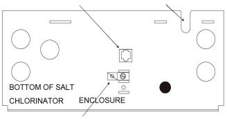
BONDING LUG TO POOL BONDING SYSTEM
