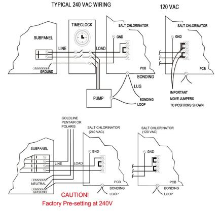
**Note:** Wire the pump directly to the time clock—do not use the salt chlorinator as a junction box.
