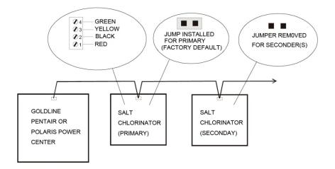
Goldline - Attach wires to proper screw terminals as show below.
