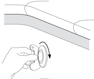
STEP 3 Using the lens wrench (part # 13.6151), thread the fixture into the wall fitting until it is snug.
