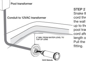
Snake the 2-conductor electric cord through the conduit outlet of the wall fitting, into the conduit and up to the location of the 12VAC pool transformer. Cut off extra cord after, allowing for service and length of run to the transformer. Pull the fixture snug to the wall
