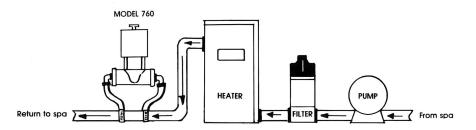
Uni-direction installation is a snap. A quality kit allows for easier installation and longer maintenance-free life.
