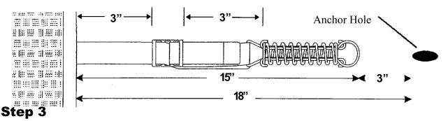
Using a hammer drill and a 3/4" drill bit, set the drill over the marked anchor holes. Keeping the drill perpendicular to the deck surface, drill down 1 7/8" into deck. This allows the anchor to lie flush with deck surface. Drilling dust should be removed from hole. Remove anchor screw from casing and spray casing and tamp tool with silicon.
