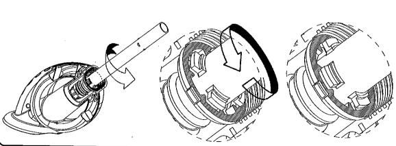
4. Push the INNER EXTENSION PIPE away from you, so the tabs go through the holes in the IEP LOCATOR.
