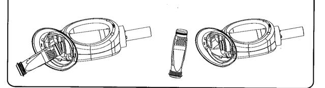
7. Remove the RETAINING RING from the DIAPHRAGM. Discard the used diaphragm.
