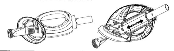
6. Twist the DIAPHRAGM, removing it from the INNER EXTENSION PIPE.
