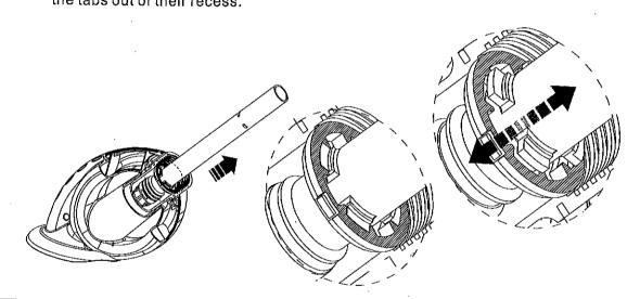
3. Turn the INNER EXTENSION PIPE so the tabs line up with the holes in the IEP LOCATOR. Do not remove the INNER EXTENSION PIPE from the BODY
