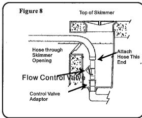
The Flow Control Valve is preset between position 3-4. This provides the ideal operating flow in most pools. But if necessary, the flow can be adjusted by using any setting from Position 1 through 6 (1= minimum flow, to slow your cleaner down, 6 = maximum flow, your cleaner will run faster). See Fig 9.
