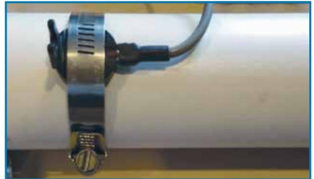
Figure 5.1. Sensor Connection
