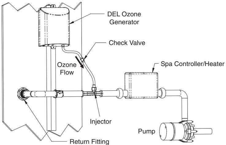
**Figure 1: Typical Injection System**
