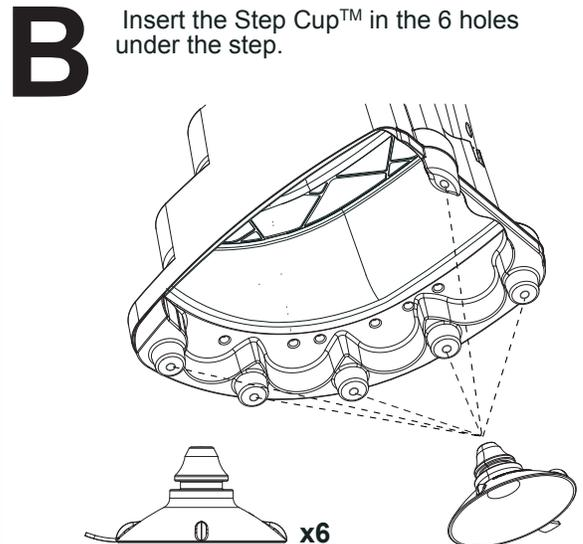
1) Insert half of the Step Cup™ mushroom in the hole, at a 45 degree angle.
