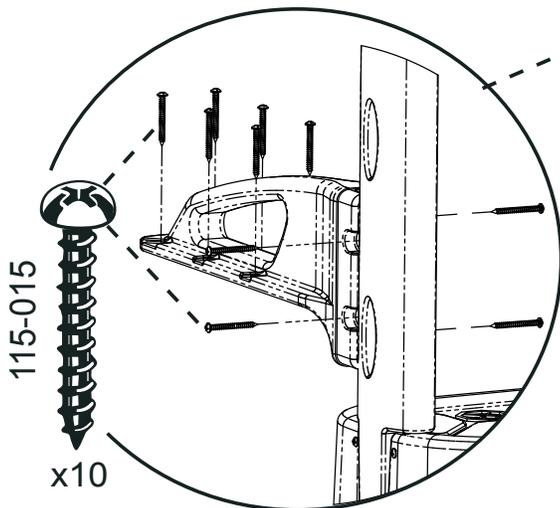
3) Align the step carefully and fasten the arm to the deck.
