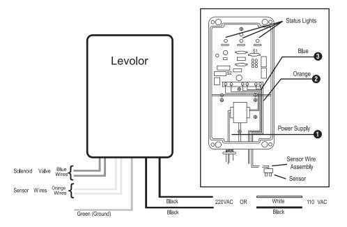
The Control Box is mounted near the Pump and Filter or in any suitable location. The LEVOLOR is available in 110VAC or 220VAC and in most cases should be wired to the load side of the time clock, this wiring method prevents the water supply from operating during unwanted hours of the day. LEVOLOR can also be wired directly to the power source for continuous operation. The controller has three (3) LED displays which illuminate to determine power on, sensor activated, and fill cycles.
