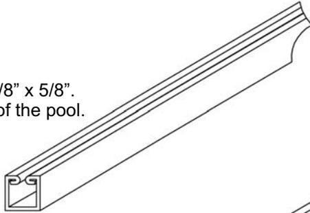
Bottom Rail 1" x 5/8". Used on the bottom of the pool.
