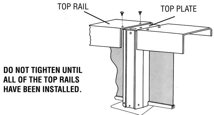
**\*USE TWO PEOPLE FOR INSTALLATION. IF A TOP RAIL FALLS INTO THE POOL, IT CAN CUT THE LINER.**
