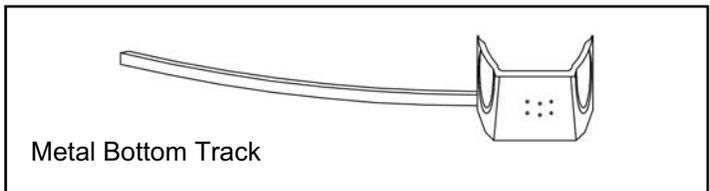
The bottom rail is inserted up to the dimple only.
