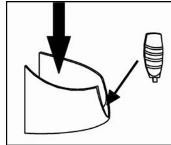
Please note the difference of the accent clips for the resin boot and the steel Upright. For proper fit be sure to use the correct clips.
