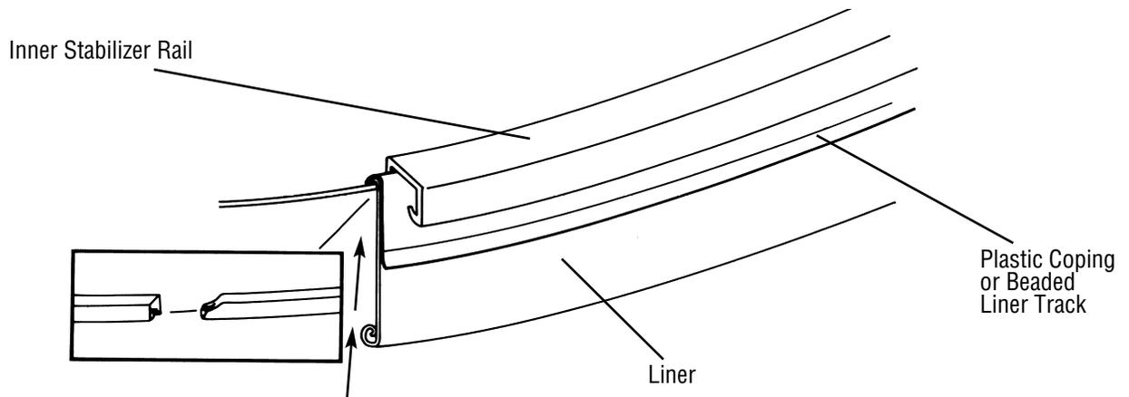
\*Roll overlap liner up inward to hide excess underneath top rail. (Rolling inward will prevent water from collecting in flap.)
