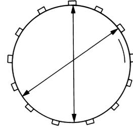
Measurements must go through center of the pool.
