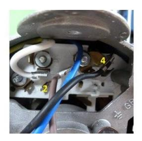
Step 7 Feed the 3 external wires through the conduit hole. Typically, the 3 external lines will be black, white and ground. These represent the hot, neutral and ground respectively.
