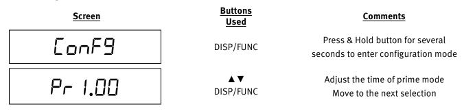
**Note:** The prime mode timer can be adjusted up to 4 minutes and down to o.oo minutes. When adjusted to o.oo minutes, prime mode will be disabled.
