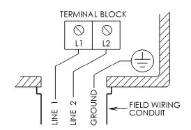
**ATTENTION:** ROUTE WIRING DIRECTLY FROM FIELD CONDUIT TO TERMINAL BLOCK AS SHOWN. DO NOT BUNDLE EXCESS WIRING INSIDE DRIVE ENCLOSURE.
