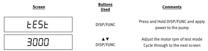
**Note:** When troubleshooting the pump it may be useful to run the pump without other program functions. This can be done in service mode. To enter service mode, remove power from the pump. Press and Hold DISP/FUNC and apply power to the pump. In this mode only the motor RPM's can be changed. To exit from service mode, cycle the power to the pump off and on.
