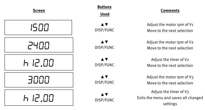
**Note:** When entering into configuration mode, the LED for the speed being configured will FLASH. When completely exited from configuration mode the LED for the speed that was currently running will illuminate. If configuration mode is not completely exited after 2 minutes, the controller will save all settings excluding the current screen settings and exit configuration mode.
