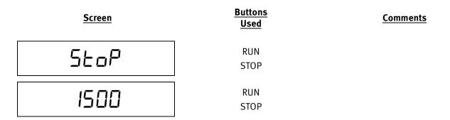
**Note:** When RUN / STOP is pressed at any time during normal operation, the above message will be displayed. The pump will stop within several seconds, and will remain stopped until RUN / STOP is pressed a second time, at which point the pump will resume normal operation.
