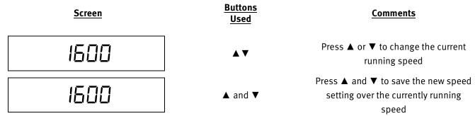
**Note:** When a quick speed change is performed the LED for the changed speed will FLASH. If the new speed setting is saved by PRESSING  $\blacktriangle$  and  $\blacktriangledown$ , the LED for that speed will illuminate solid. If the new speed setting is not saved, the pump will continue to run at the changed speed until the timer runs out for that speed or the speed is changed again. The LED for the changed speed will FLASH as long as a modified speed is running and has not been saved.
