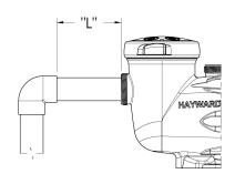
**\* Note:** It is recommended that a minimum length of straight piping (shown as "L" in above diagram), equivalent to 5 pipe size diameters, be used between the pump suction inlet and any plumbing fittings (elbows, valves, etc.).
