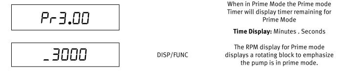
Note: When Pump has finished Priming the pump will start speed V3 and display RPM.
