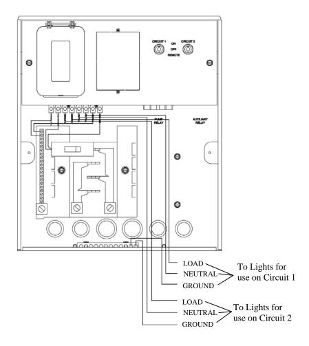
If this product is used to connect underwater lights directly, refer to 1999 NEC 680-21(b), 2002 NEC 680-24(b) or CEC 68-060, 062 and 066 for details.
