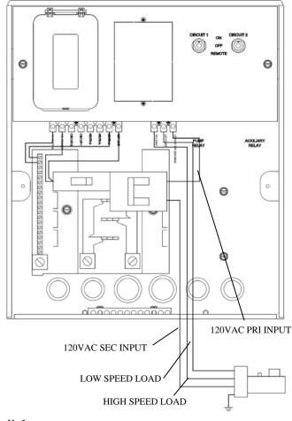
Note: Circuit 2 is pre-wired. There is no connections or external wiring.
