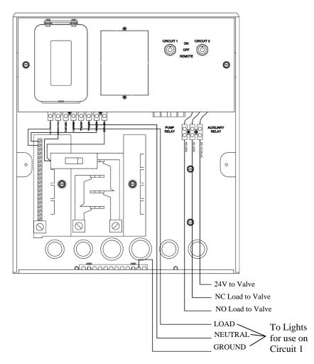
If this product is used to connect underwater lights directly, refer to 1999 NEC 680-21(b), 2002 NEC 680-24(b) or CEC 68-060, 062 and 066 for details.
