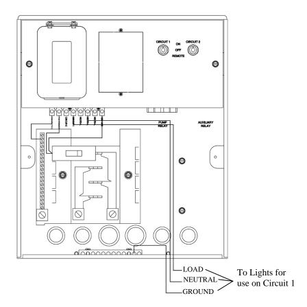
If this product is used to connect underwater lights directly, refer to 1999 NEC 680-21(b), 2002 NEC 680-24(b) or CEC 68-060, 062 and 066 for details.
