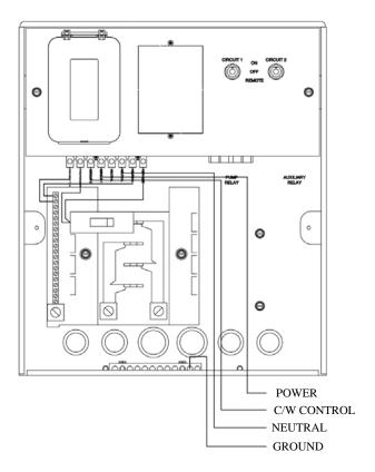
If this product is used to connect underwater lights directly, refer to 1999 NEC 680-21(b), 2002 NEC 680-24(b) or CEC 68-060, 062 and 066 for details.
