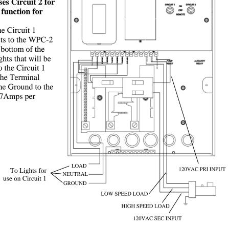
NOTE: Pump Breaker MUST be turned OFF before servicing as  $2^{nd}$  leg of 240V circuit is HOT at all time!
