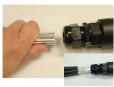
While holding the ferrules together, insert into the strain relief opening as illustrated.
