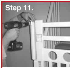
Install the latch to the upper mounting block of the latch mounting post using four (4) #10 x 1-1/4" self tapping screws.
