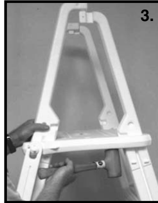
Tap upward on ladder deck/platform.
