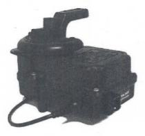
Mount Valve Actuator to solar valve using the 4 mounting screws provided. Run cable to solar control. Loosen LOCK SCREW on service panel of Solar Control, and swing open to expose the high voltage and low voltage compartments. Insert Valve Actuator cable through hole on bottom left side of Solar Control, and plug into circuit board at VLV1 socket.
