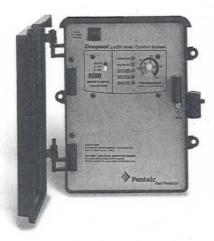
Select a convenient location to mount the Control, making sure that the location is greater than 5 feet from the Pool or Spa and no further than 15 feet from the Solar Valve. Wall-mount the Control, using appropriate screws through the three external mounting points located on the side of the enclosure.
