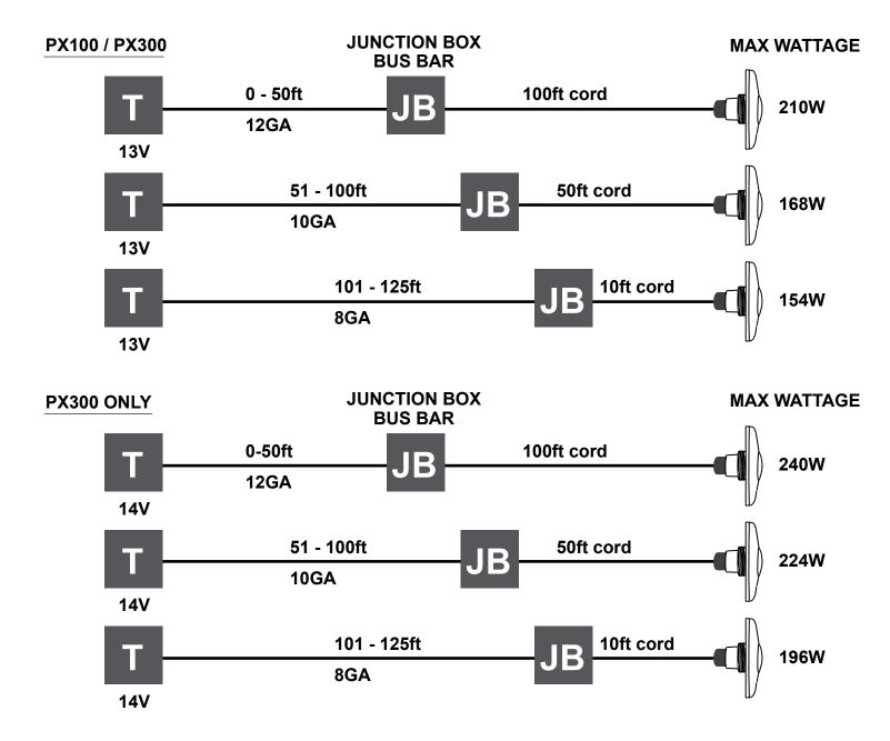
NOTE: Please use appropriate low voltage supply to pool lights, ie. if 12V is appropriate voltage do not use 13V or 14V tap on transformer output.
