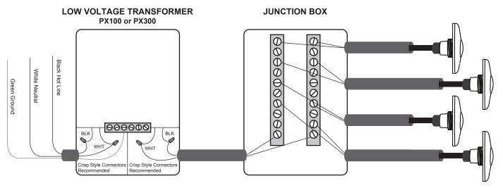
**NOTE:** This Diagram is to be used as a guide line only for a typical System Installation and should only be used as such. It is the Installers sole responsability to varify and assure that proper gauging of secondary wiring from the Transformer to the J-Box are in compliance with your local. State and National Electrical Codes.
