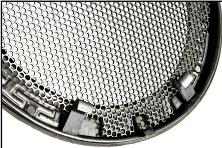
4. Place the bottom of the screen into the face ring aligning the feet around the tab. Note that the smooth beveled side of the screen should face outward toward the front of the face ring.
