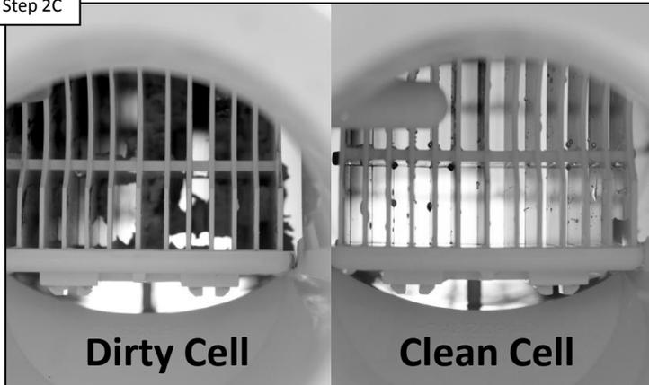
The TurboCell must be clean to report accurate salt readings. IF the cell looks like the image on the left, then clean the cell ([pg.13-15](#)). IF cell is clean, proceed to step 2D.
