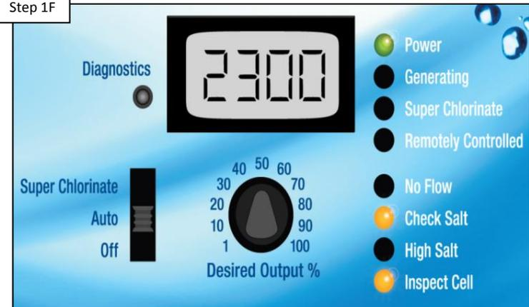
IF the "Check Salt" & "Inspect Cell" LEDs cleared, then the problem is solved. IF not please contact technical support directly by dialing: 908.355.7995 or email support via [Hayward.com](http://Hayward.com)'s support page.
