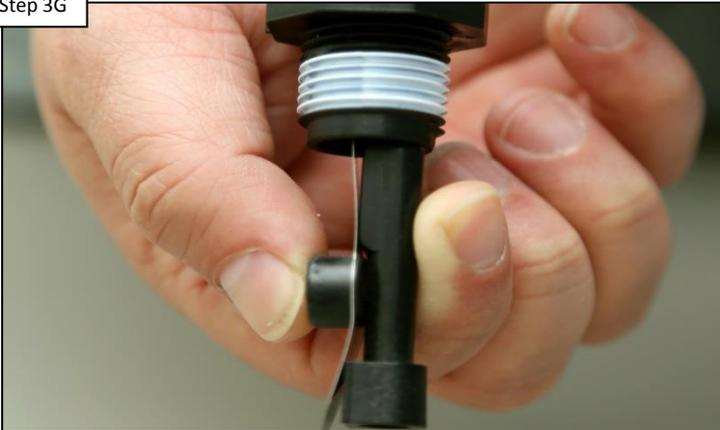
**Plug a confirmed (working) Flow Switch into the control center and hold it closed, manually, for 60 seconds. Monitor the “No Flow” LED. IF LED goes out, install this new switch. IF LED remains on go to step 3G.**
