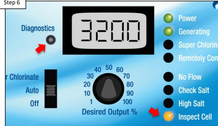
IF the "Inspect Cell" LED was flashing alone, press and hold the diagnostics button for 5 seconds OR until the Inspect Cell LED goes out. This will reset the inspect cell timer for another 500 operational hours.
