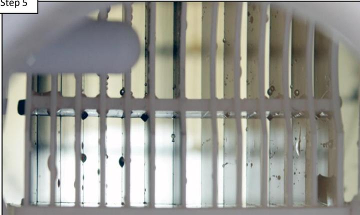
After the solution has been safely removed, thoroughly rinse the TurboCell before returning it to its place in the plumbing. Once returned turn the pump back ON and proceed to the step 6.
