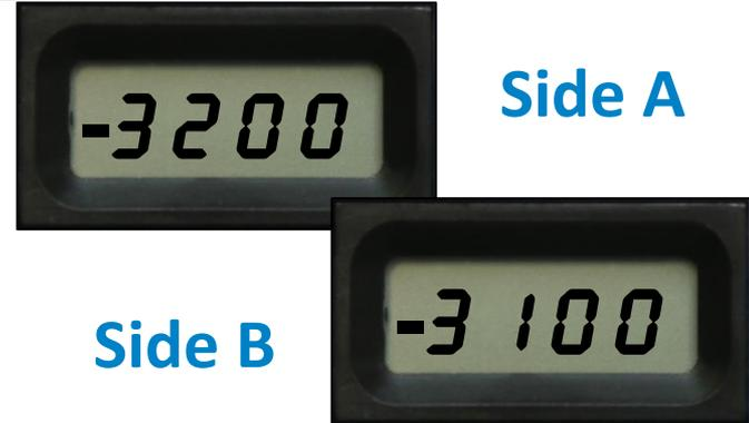
Reset the average salt level, twice, following the steps on [pg. 11](#). Are the two instant salt level readings within 500ppm of each other? IF not go to step 2E. IF they are go to step 2F.
