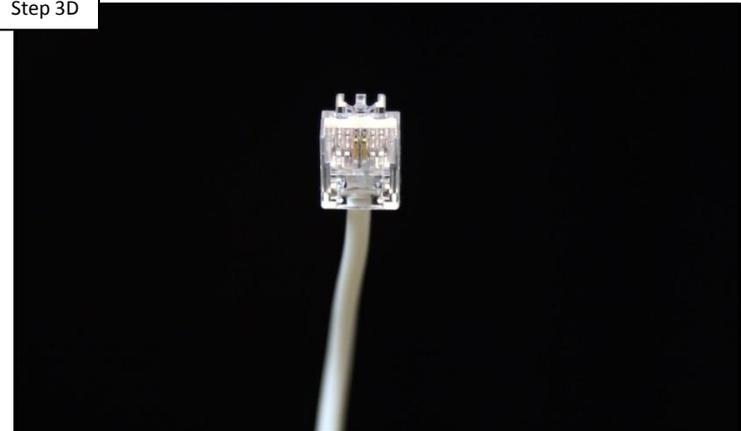
Unplug the flow switch connector & inspect. Plug the connector back in, waiting 60 seconds. IF connector is damaged, replace flow switch (GLX-FLO-RP). IF connector is not damaged, proceed to step 3E.
