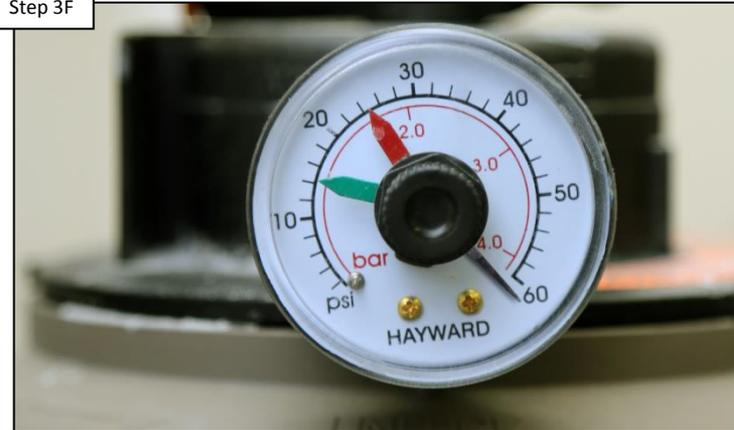
**Check Filter pressure & pump basket for debris. Remove debris, backwash / clean filter. Turn pump ON & wait 60 seconds. IF LED is still ON go to 3G.**
