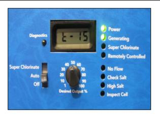
To switch Cell Type, cycle Main Switch from AUTO → Super Chlorinate → AUTO.
