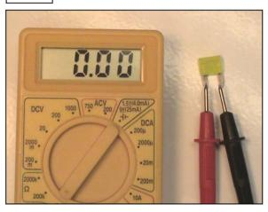
Replace fuse if blown. If fuse OK, go to step G.
