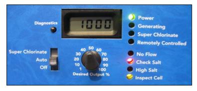
NOTE: Check Salt & Inspect Cell LED's will also be ON if the control is set for the wrong Turbo Cell type or the cell is unplugged.
