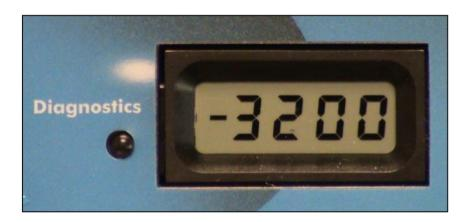
Press Diagnostics button 5 times to display Instant Salt level. Wait for the number to settle.
