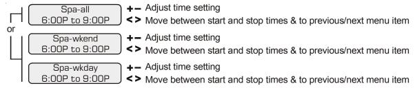
This menu is only available if the system has been setup for "pool and spa-std". During the programmed spa time, the Aqua Plus 16v will move the pool/spa valves into the "spa-only" position and turn on the filter pump. The heater will automatically heat the spa up to the programmed spa temperature. This programmed spa operation will take precedence over all other automatic functions, only manual operation of the filter button or pool/spa valve button will override this function.
