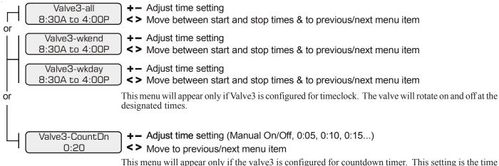
after you manually turn on the valve3 relay until the Aqua Plus 16v automatically turns off the relay. You can also manually turn off the valve at an earlier time by pressing the VALVE3 button.
