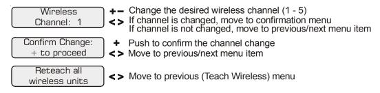
This setting changes the channel to be used by the wireless base station and remote(s). If the channel is changed and confirmed, all wireless remote will have to be re-taught. This menu will only appear if a wireless base station is connected to the Aqua Plus 16v.
