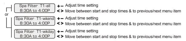
This menu is only available if the system has been setup for Dual Equipment. For one speed pumps, this is the first spa filter timeclock and will determine the normal hours of filtration for the spa. For pool/spa combination systems with spillover enabled, the valves will automatically switch to pool only at the start of the filtration period.
