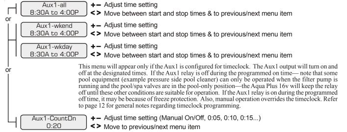
This menu will appear only if the Aux1 is configured for countdown timer. This setting is the time after you manually turn on the Aux1 relay until the Aqua Plus 16v automatically turns off the relay. You can also manually turn off the relay at an earlier time by pressing the AUX1 button.
