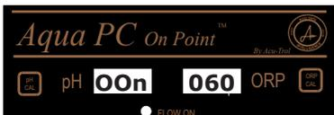
This menu will allow the user to select the amount of time in seconds that the Aqua PC On Point will feed ORP sanitizer each time the controller calls for ORP chemicals. The default ORP On Time is 60 seconds.
