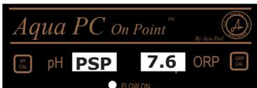
The pH Set Point menu should now display the desired setpoint. Press the Save/Exit button to save the changes and return to the readings screen.
