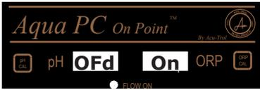
The ORP Feed Menu display should now read On. Press the Save/Exit button to turn on the ORP feed system and return to the readings screen. Do not manually feed pH and sanitizer at the same time. Manual ORP feed will not allow ORP chemicals to feed if there is no flow in the system
