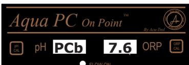
The Calibrate pH menu display should now be the same as the manual reading. Press the Save/Exit button to save your changes and return to the readings screen.
