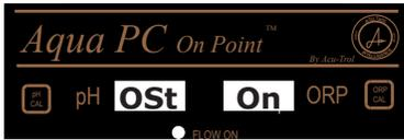
The *Aqua PC On Point* has the ability to automatically turn off the ORP feed system once the current reading is equal to the set point. This helps to prevent overfeeding and makes it easier for the controller to reach the exact set point.
