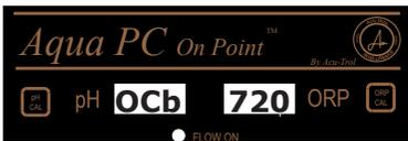
The Calibrate ORP menu display should now be the same as the manual reading. Press the Save/Exit button to save your changes and return to the readings screen.
