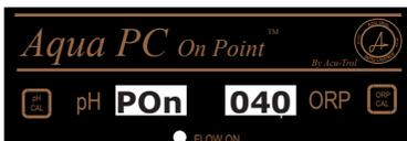
The pH On Time menu should now display the desired on time. Press the Save/Exit button to save the changes and return to the readings screen.
