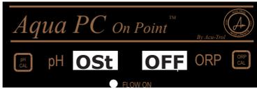
The controller will now automatically turn off the ORP feed system when set point has been reached. Press the Save/Exit button to save your changes and return to the readings screen.
