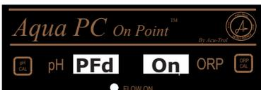
The pH Feed Menu display should now read On. Press the Save/Exit button to turn on the pH feed system and return to the readings screen. Do not manually feed pH and sanitizer at the same time. Manual pH feed will not allow chemicals to feed if there is no flow in the system.
