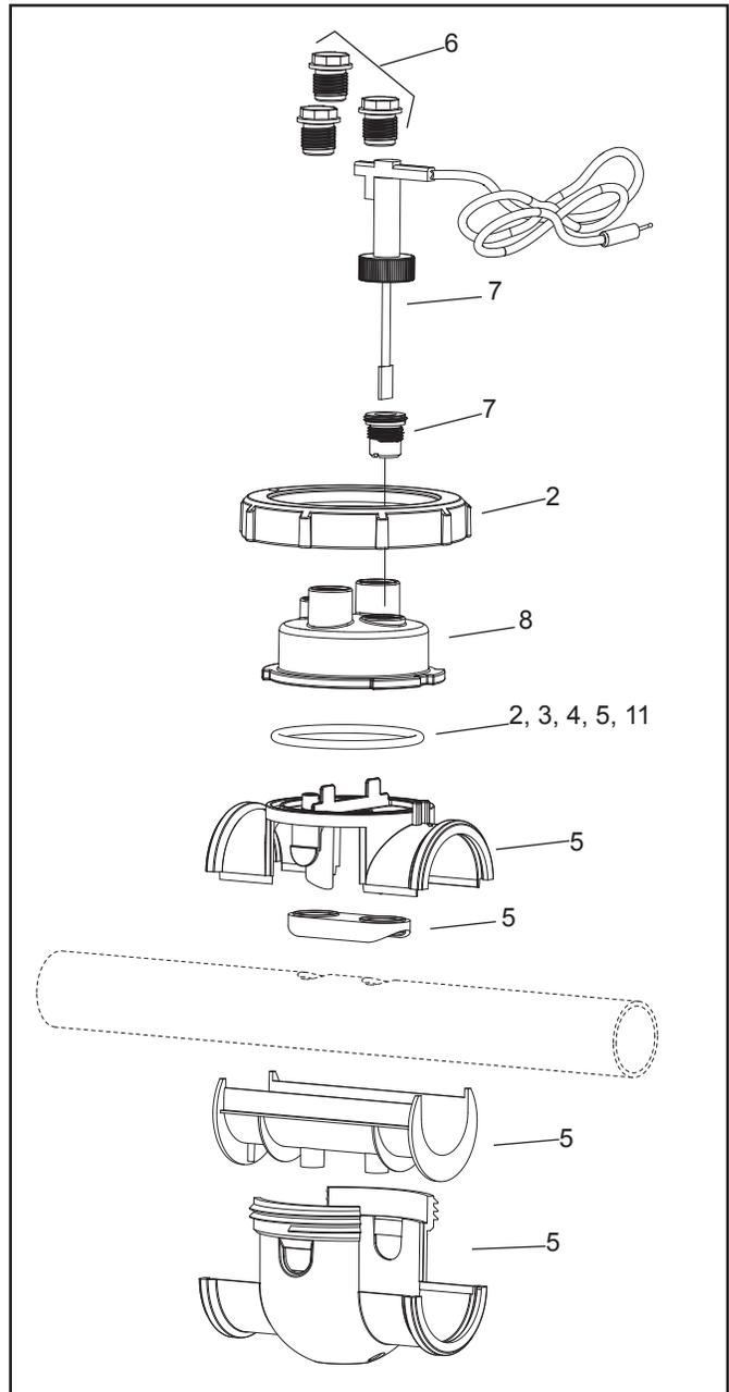
Figure 30. Pod Exploded View
