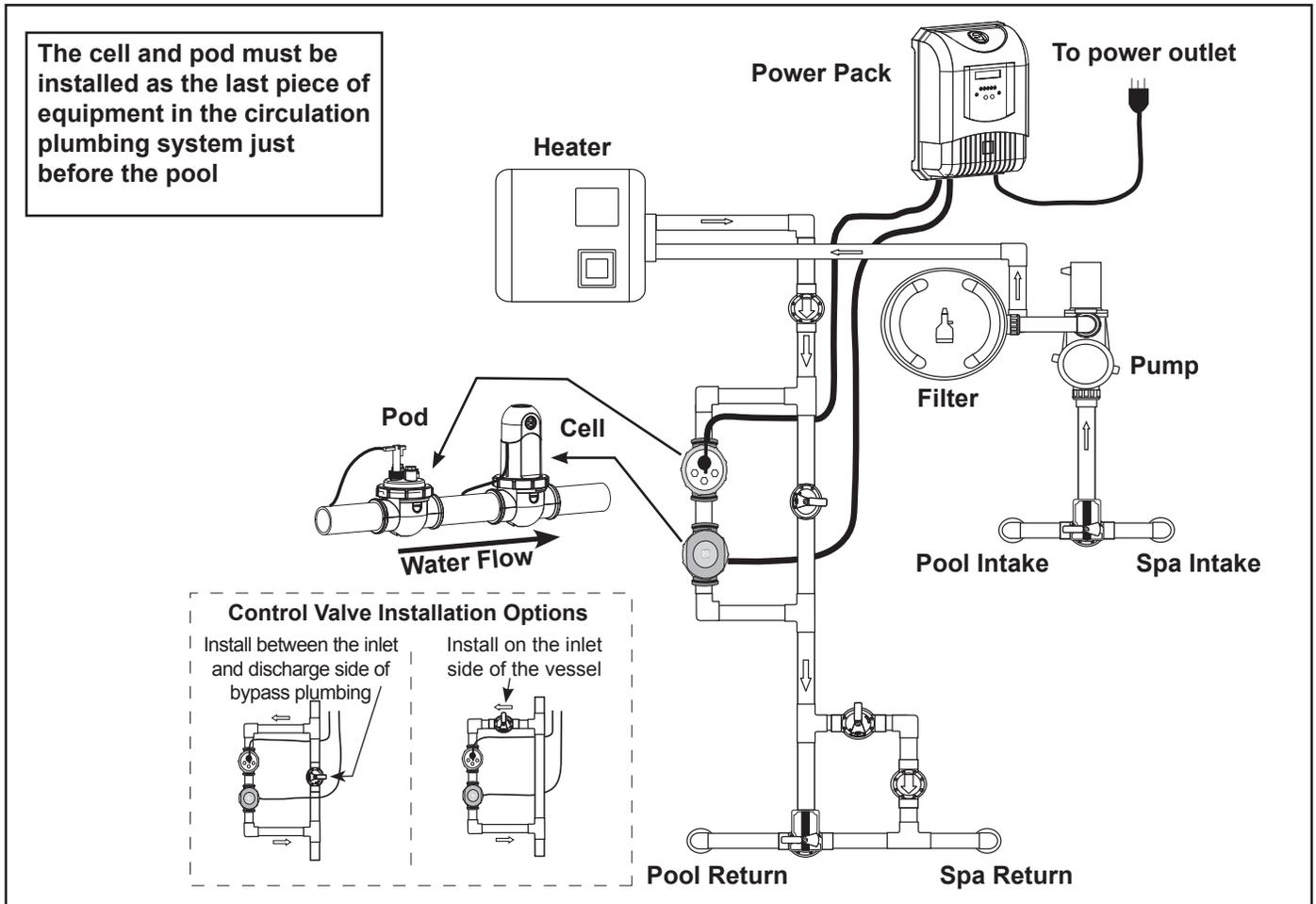
Figure 19. Example of Bypass Installation
