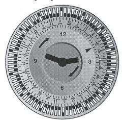
To set the time of day: rotate the entire dial until the clock indicates the correct time of day.
