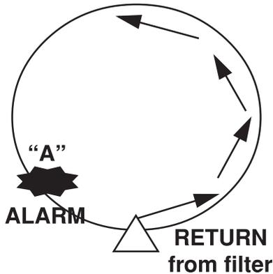
If the water returning from the filter is positioned at 6 o'clock and the flow is counterclockwise, the best location to put the alarm is between 8 o'clock to 9 o'clock - position "A".
