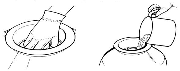
4. Take away the funnel, and then clean really carefully the tank's neck and fix the valve with O-ring through flange clamp set. (the direction of "PUMP" port on valve needs to face pump out port)
