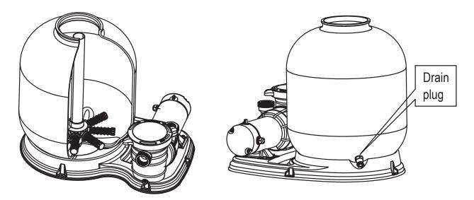
3. Insert the tube with the diffuser body inside the tank as above picture, then place the funnel on the tank's mouth and pour the quartz sand into the tank (sand weight 85kg).
