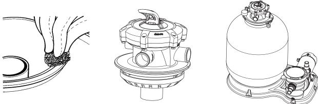
5. Connect the sand tank to pump with hose, hose clamps and hose adaptors.
