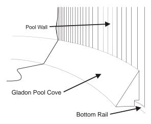
Step 8 Cut the last piece of cove about 1½ inches longer than the remaining space. Use a fine tooth saw to cut the cove, keeping the cut as square as possible. Insert the final piece of cove into the pool bottom rail. This tight fit will compensate for the wall stretch that will occur when your pool is filled with water.
