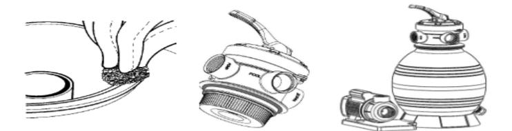
5. Connect the sand tank to the pump with the pump hose, hose clamps, and hose adapters.
