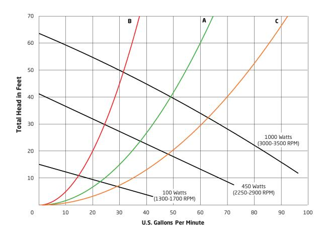
*B*, *A*, and *C* represent average system curves for pools with the pipe diameter mentioned below.
