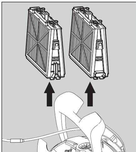
**9.1.1** Open the filter covers and remove the cartridges from both sides of the robot.
