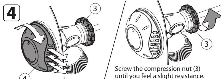
Screw the compression nut (3) DO NOT TIGHTEN. Position the the Dome (4) to direct the water flow.
