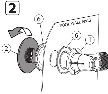
Screw the wall plate (2) into the main body (1) trapping a wall gaskets (6) on each side of the pool wall. Hand tighten the wall plate keeping the main body with the water inlet horizontally to the right.
