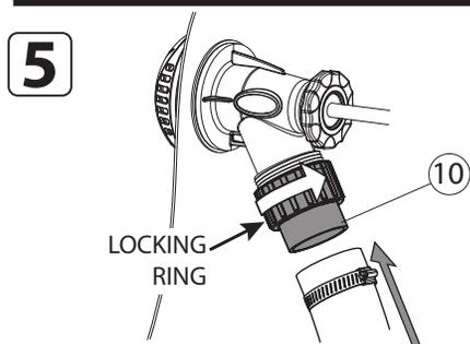
Choose your union (10) and screw it onto the main body (1) with the locking ring. Connect or glue, your inlet hose.
