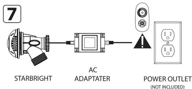
Install your AC adapter preferably sheltered from the elements. Connect the light to your AC adapter. Read the following instructions before connecting to power outlet.
