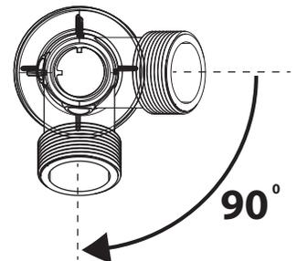
Once the wall plate (2) is tight, complete by holding the wall plate and turning the main body 90 degrees as shown.
