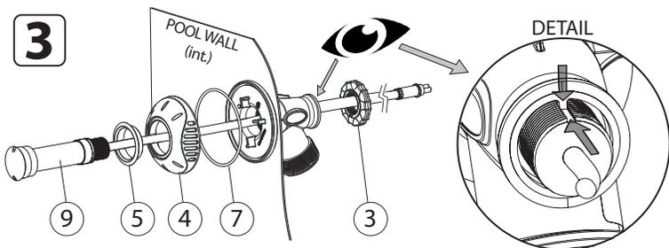
Assemble the remaining parts (9,5,4,7,3). Be careful to align the main body's key (1) onto the light's (9) keyway. See detail
