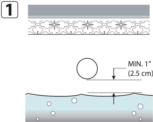
The water level of your pool must be at least 1 inch below the opening on your pool's wall. Disconnect the water inlet hose from the inlet fitting. Completely remove the inlet fitting. At this point, the hole on your pool wall is all that remains.
