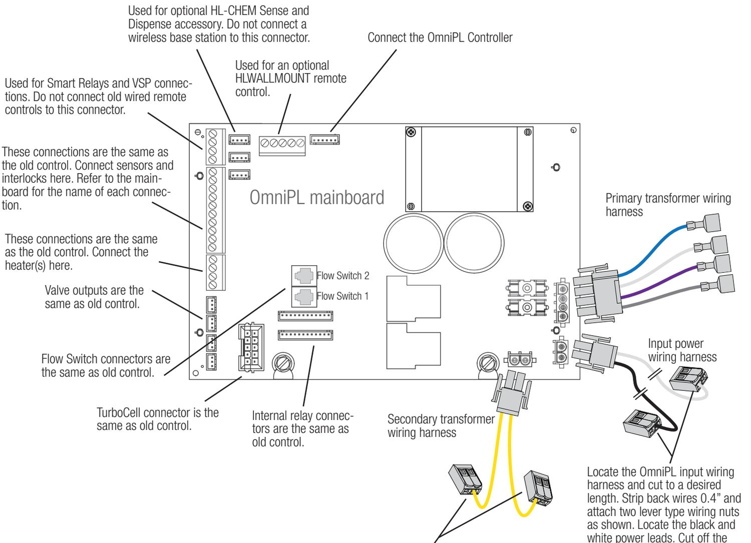
The OmniPL secondary transformer wiring harness included in the kit plugs it into the mainboard as shown. Strip back wires 0.4" and attach two lever type wire nuts according to the diagram above. Locate the two yellow leads from the transformer secondary (refer to Step 3). Cut off the spade connectors and strip wires back 0.4". Insert stripped bare leads into the wire nuts and close the levers to secure. Be sure that no bare wire can be seen coming out of the wire nuts.
