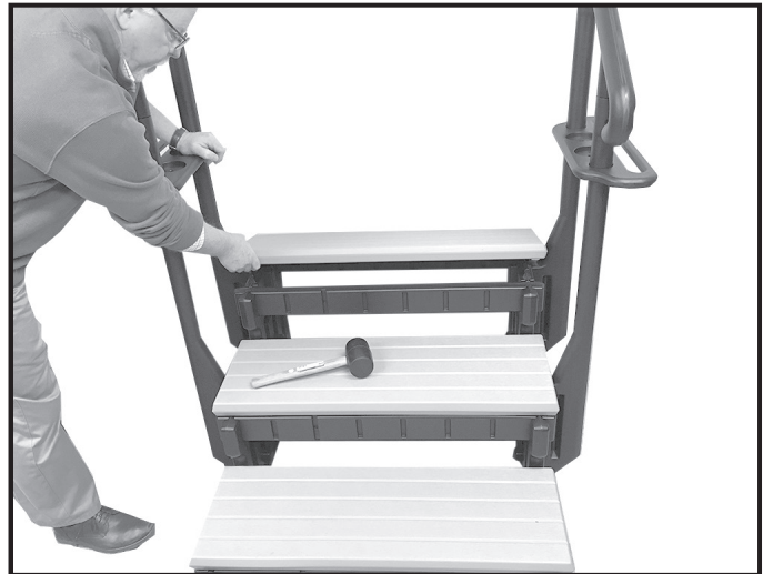
Step 10: Install the steps (finished edge out) by placing over the male lugs on the step sidewall and hitting downward with a rubber mallet.
