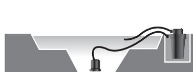
D. Below ground, pumped up to the pond.
