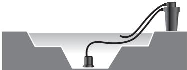
A. Above ground, pumped back into pond.
