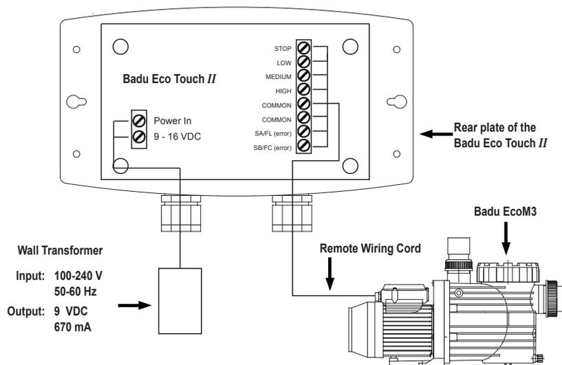
**NOTE: If the Badu EcoM3 has an STOP switch the wiring is as follows:
