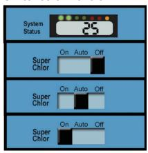
**AUTO:** Generally, if the Crystal Pure is in "Auto", it will automatically work according to the chlorine output settings.
