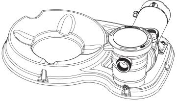
2. Place the tank onto sand filter support with correction direction (drain plug is at outside as below picture).
