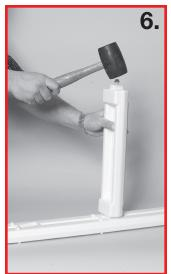
Push the end of one of the standard treads into the uppermost keyhole slot. Make sure that the tread and the ladder leg are positioned as shown in the photograph to the left. It may be necessary to tap the tread into the slot with a mallet. Repeat for three additional treads.
