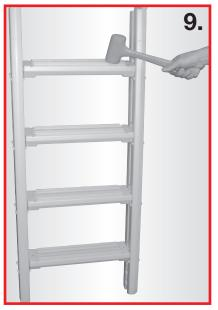
With the ladder standing up, tap the treads all the way down until seated in the keyhole slots
