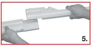
Place handrail over the flat area located on top of ladder leg. Insert one of the  $1/4 - 20 \times 1$ " bolts through the ladder leg into the handrail. Place one 1/4 - 20 hex nut into the recessed area on the handrail and tighten using a Phillips screwdriver. Install the second bolt and nut. Repeat to assemble all four ladder leg/handrail assemblies.
