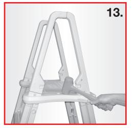
Tap the platform down until fully seated on the lugs as shown.
