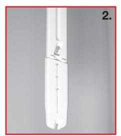
Slip the four extension boots over the ends of the ladders legs. They will need to be all the way on for most 52" tall pools and backed off one hole for 54" pools. Depending upon ground levels outside the pool, and sand levels under the liner inside the pool, a final adjustment may need to be made after the ladder is put into place.
