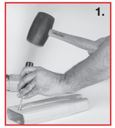
If the round plastic inserts, on the sides of the extension boots, are still in place, remove them with a phillips head screwdriver as shown.
