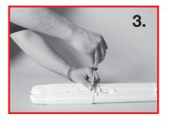
Using four 1/4-20 x 2" long bolts and four acorn nuts fasten the extension boots to the ladder legs
