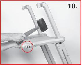
Making sure that the "swing-up" side of the platform is facing away from the "inside" ladder section, as shown, slip the openings of the platform over the upper ends of the ladder legs. Using a mallet or hammer tap the platform down until it is fully seated onto the "nubs" of the ladder legs. Liquid soap or lubricant will help the parts slide together.
