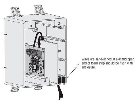
Install the cover back on to the enclosure and power on the Omni Control and Pentair pump(s). Proceed to Operation.
