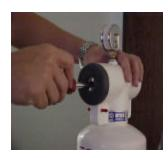
• With a flat head screwdriver turn the adjustment screw (3) full revolutions to the right (clockwise), reset the piston by pressing down the reset lever, and restart the pump. Check for an air leak. If an air leak persists, lock open the piston, and repeat this procedure until air no longer leaks through the vent end of the SVRS unit.
