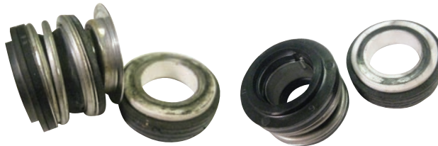
PTFE or Silicone Based Lubricants Destroy Seals
