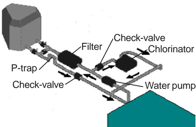
The pressure-type chlorinator or brominator takes a small amount of water from the outlet side of the filter, adds chemicals to it and returns this highly concentrated solution to the pool. The check valves must be highly resistant to corrosion. Use only a check-valve either supplied or recommended by the chlorinator (brominator) manufacturer.
