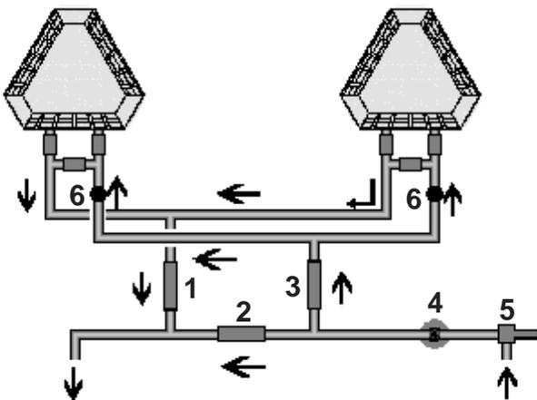
For some larger pools, it may be necessary to install two units in parallel. In this case, double the distances recommended in the table 1 of the page 5. Never place two MP models coil against coil, fan against fan or coil against fan.
