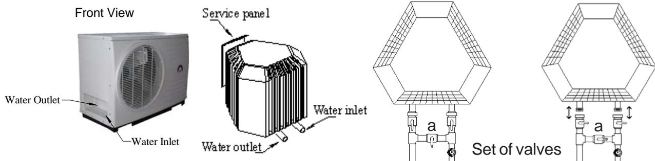
To adjust the water flow going through the pool heater, please adjust the by-pass valve (a) in the following way:
