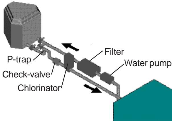
The in-line chlorinator or brominator should be installed on the pool water return line, between the heat pump and the pool. This type of chlorinator (brominator) should be installed as far as possible from the heat pump. Install a check-valve between the heat pump and the chlorinator (brominator).
