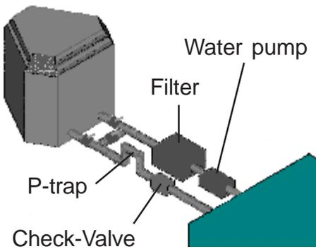
This connection method is strongly recommended to enhance the life-span of your pool heat pump.
