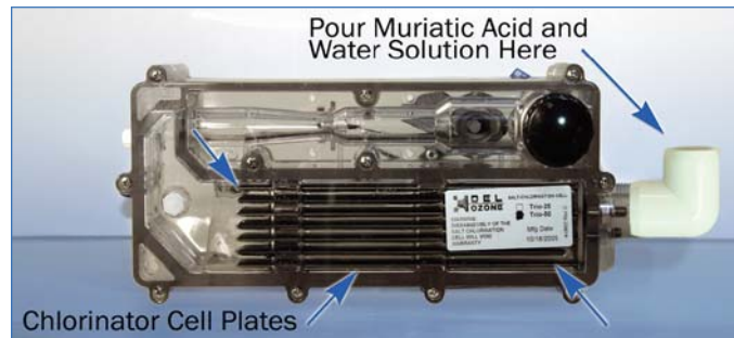
Figure 24 - Chlorinator Cell Plate Cleaning
