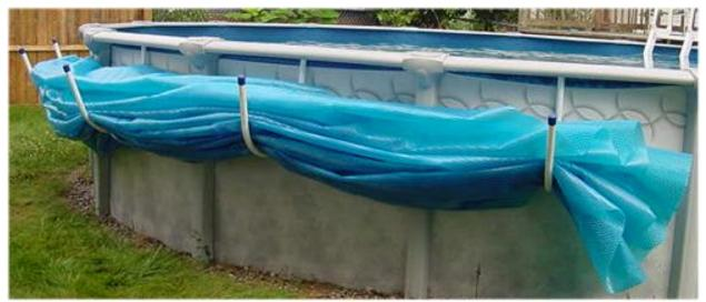
The key to mounting the accessory is to evenly space the saddles to allow 2-1/2 to 3 feet of the cover to extend over/past the outside holders, which will vary with different size pools. Refer to the picture above which shows the Solar Saddles mounted on a 27 foot round pool and the solar cover stored neatly in the Solar Saddles.
