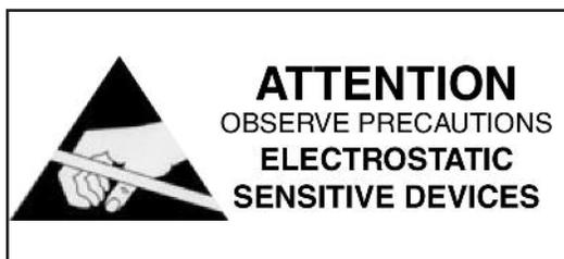
**Note:** Electrostatic Discharge (ESD) damage can be caused by direct or indirect contact with the wiring or circuit board. When one walks to the heater area, an electrostatic charge accumulates on the body. Contact of a finger allows the body to discharge, possibly causing device damage. This damage can be limited if the service person discharges himself, following ESD preventive/removal practices, and holds on to the heater enclosure for 5 seconds before proceeding.
